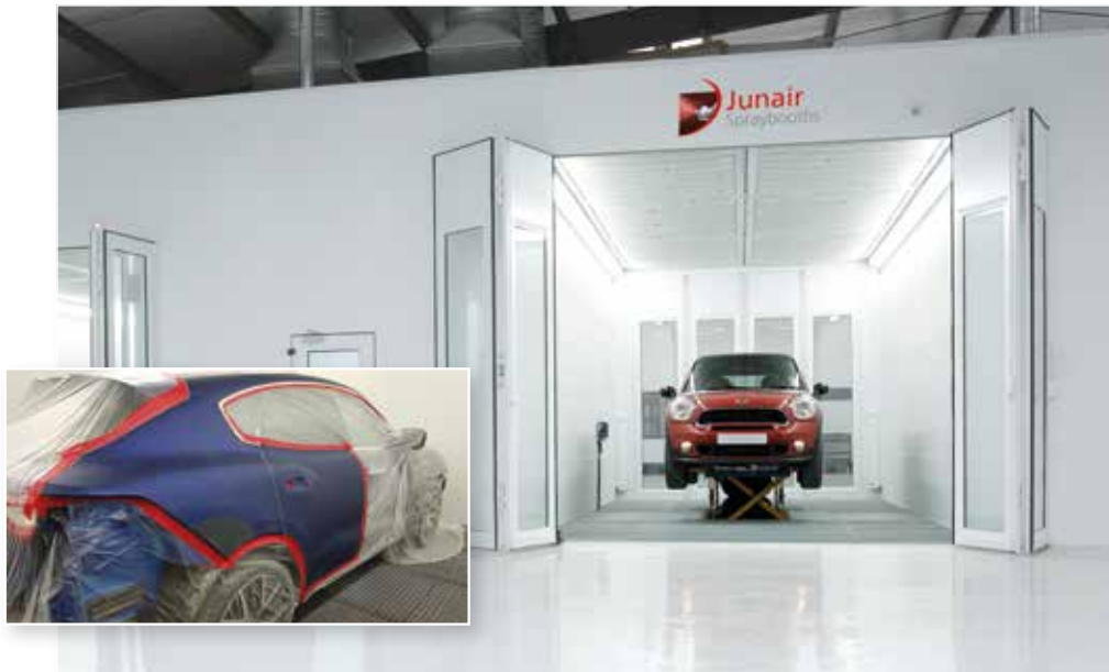
▲ Automotive spraybooth - downdraught for excellent airflow
